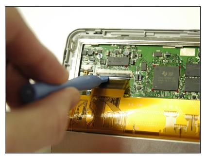
Use a plastic opening tool to get underneath the black flap on the larger ribbon cable connection and lift it.
