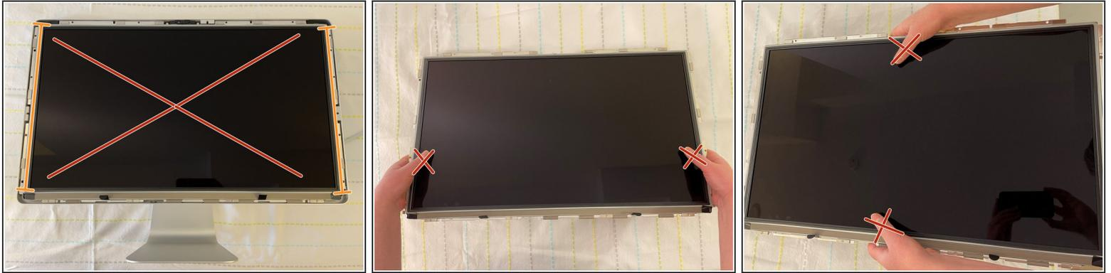
**i First Steps** Remove the glass panel as shown on step 2.
