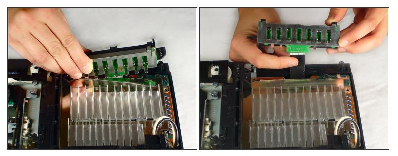
• Gently lift the controller port board out of its recess within the bottom case.
