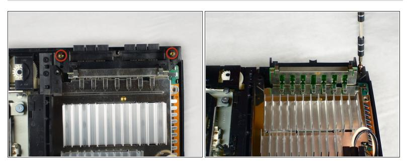
• Remove the two 14.6 mm gold-headed Phillips securing the controller ports to the bottom case.
