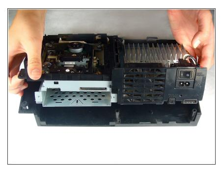
• Lift the motherboard assembly from its front edge and remove it from the lower case.
