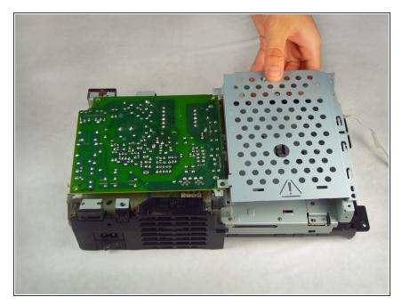
• Lift the expansion bay cage up off the motherboard assembly.
