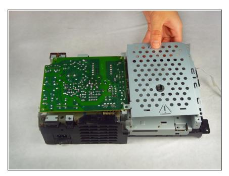
Lift the expansion bay cage up off the motherboard assembly.
