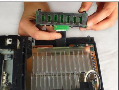
Gently lift the controller port board out of its recess within the bottom case.
