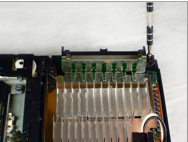
Remove the two 14.6 mm gold-headed Phillips securing the controller ports to the bottom case.
