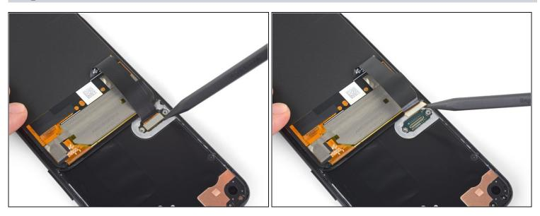
• Use the tip of a spudger to pry up and disconnect the screen flex cable.
