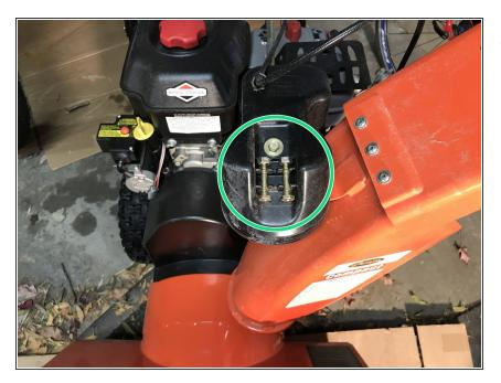
The new shear bolt is stored on the top of the auger discharge
