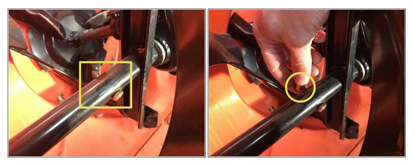
• With the new bolt in place from pushing the old bolt out add a nut
