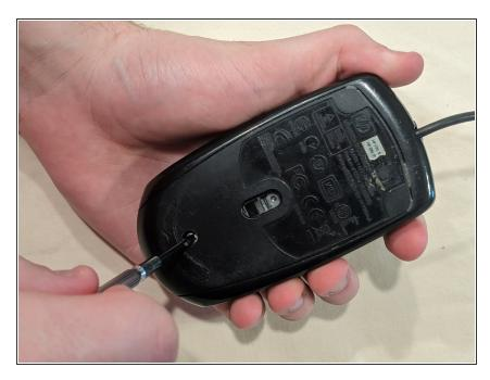
Flip the mouse upside down and remove the screw on the bottom of the mouse casing using a Phillips #00 screwdriver.
