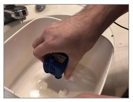
Remove the pump from the fountain by grabbing both sides of the pump and the basin, then pulling the pump out.
