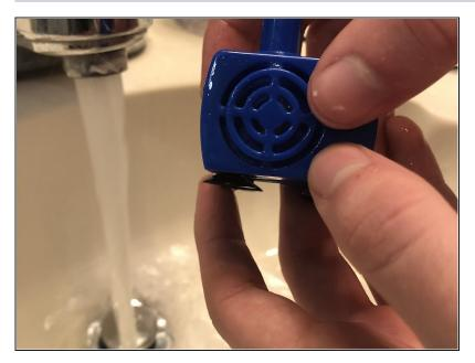
Take the front face plate and place it onto the pump. You should hear a snapping sound when face plate is fully on. The snapping sound comes from the tabs on the front face place popping back into place.
