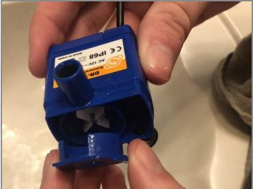
• To remove the inside cover pull on the tab shown in the picture.
