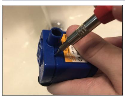
Take your flathead screwdriver and pry along the seam of the front face plate of the pump. Once it is loosened, pull it off with your hands.
