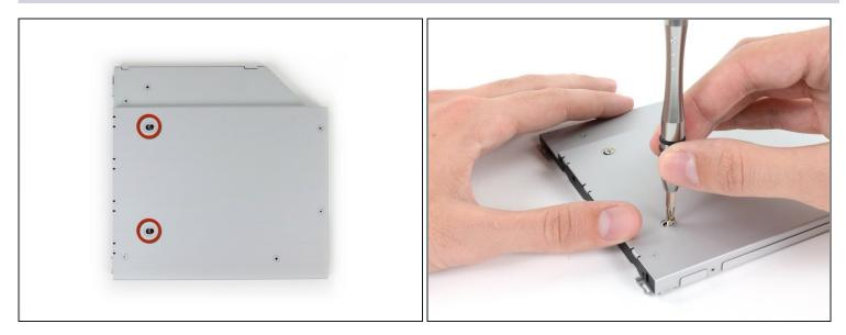
• Use two Phillips #1 screws to secure the drive to its enclosure.
