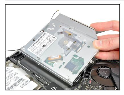
• Pull the optical drive upward from its edge closest to the display and remove it from the upper case.
