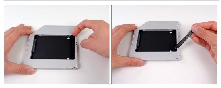
• Remove the plastic spacer from the optical bay hard drive enclosure by pressing in on one of the clips on either side and lifting it up and out of the enclosure.
