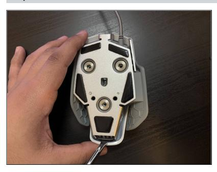
There are 2 screws in the base of the M65 elite, either side of the lowest weight screw. Use a long Phillips PH00 to remove these, as they will make removing the inside cover easier
