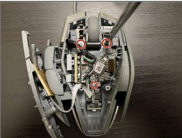
Remove the three 2 mm screws attached to the PCB using a Phillips screwdriver.
