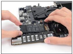
To avoid damaging its socket, do not lift the end of the SSD above about 15°.
