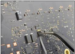
• Use the tip of a spudger to flip open the retaining flap on the microphone ribbon cable <u>ZIF socket</u>.
