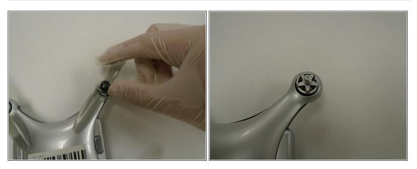
Holding the base of a propeller with one hand, unscrew the propeller by hand in a clockwise direction. Complete this action on all 4 propellers.
