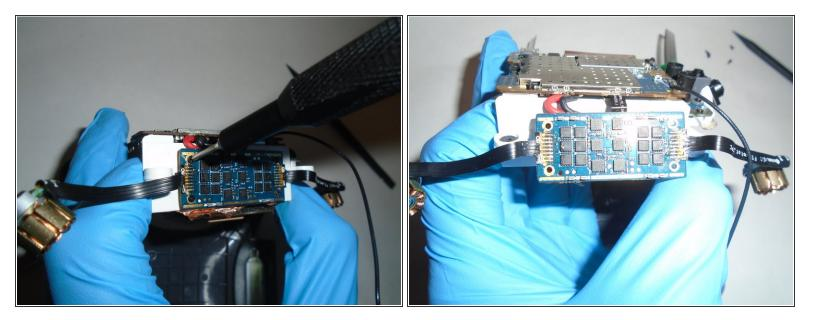
Using a Phillips #00 screwdriver, remove the four screws separating the side board from the white chassis.
