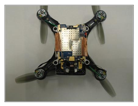
Using a Phillips #00 screwdriver, remove the screws from the four corners of the inner white chassis.
