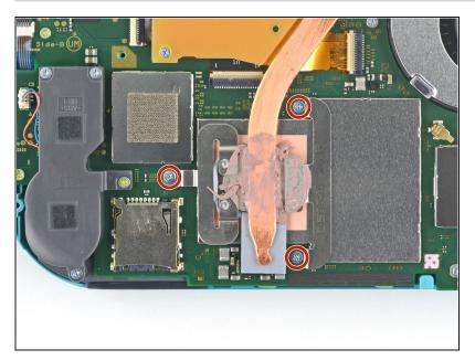
Use a JIS 000 driver or an official iFixit PH 000 driver to remove the three 3 mm screws securing the heat sink to the motherboard.
