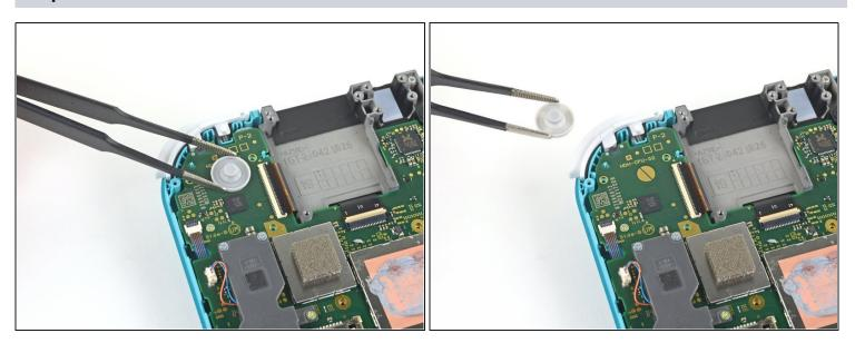
Use a pair of tweezers or your fingers to remove the right trigger button assembly's rubber pad
