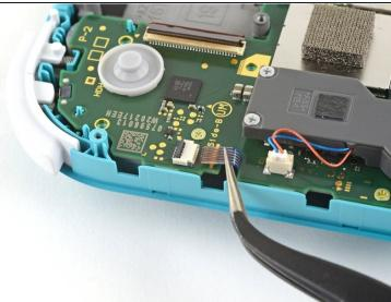
• Use a pair of tweezers to slide the right joystick cable out of its connector on the motherboard.
