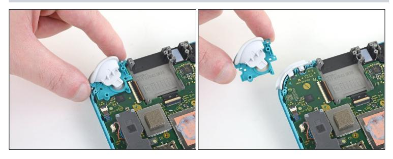
Remove the right trigger button assembly.
