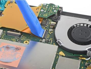
Use an opening tool or your fingernail to flip up the small, hinged locking flap on the game card reader cable's ZIF connector.
