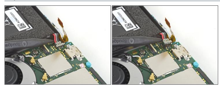
Use the point of a spudger to pry the battery connector straight up and out of its socket on the motherboard.
