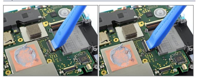
• Use an opening tool or your fingernail to flip up the small, hinged locking flap on the screen cable's ZIF connector.
