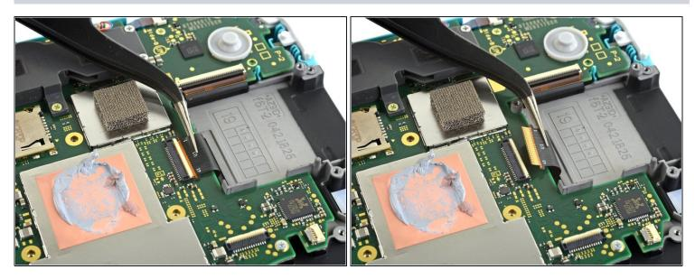
• Use a pair of tweezers to slide the screen cable out of its connector on the motherboard.
