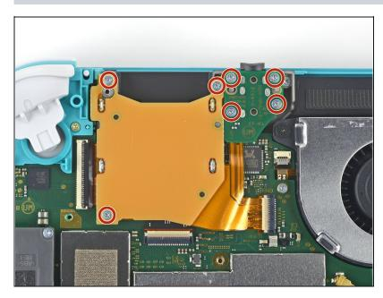
Use a JIS 000 driver or an official iFixit PH 000 driver to remove the seven 3.1 mm screws securing the game card reader and headphone jack.
