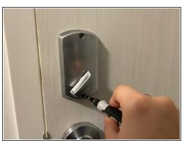
Remove the two 3 mm Phillips #1 screws from the battery cover.
