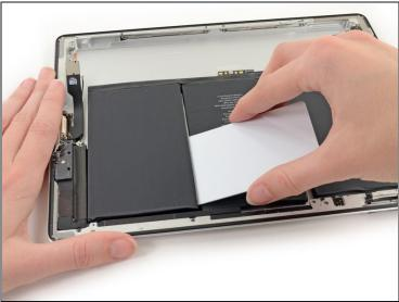
• Gently pry the corner of the battery off of the case to begin freeing the final side of the dock side cell.
