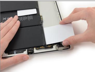
• On the battery cell nearest the headphone jack, run a second plastic card underneath the edge adjacent to the logic board void.
