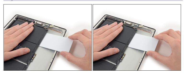
• Starting with the battery cell closest to the dock connector, run a plastic opening tool underneath the edge of the battery closest to the logic board void to make enough room to insert a plastic card.
