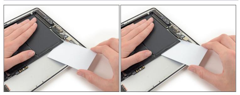
• Insert the card at the case side corner and slide inward to separate more adhesive.
