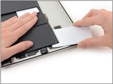
• Slide the card in to free the corner of the cell from adhesive.
