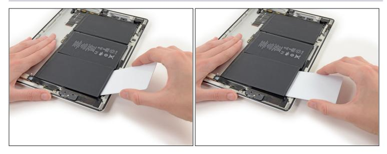
• Gently pry the end of the battery cell away from the case.
