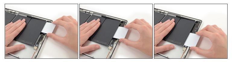
• Slide the card along the side of the cell to detach any remaining adhesive.
