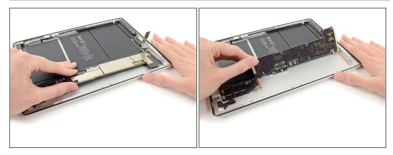
• Lift the logic board out from the rear case and flip it over toward the battery.
