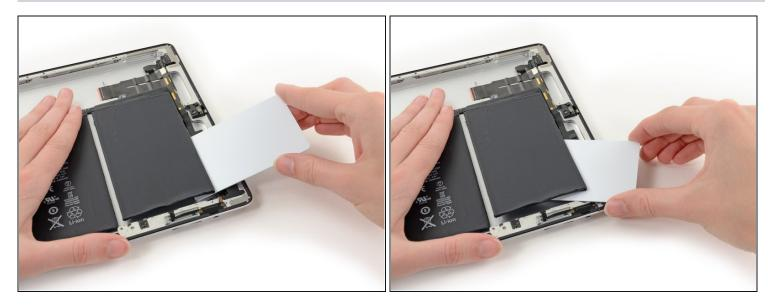
• A final pry, and the card can be left in place to keep the battery propped away from the adhesive.
