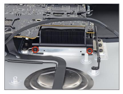
Use a T8 Torx screwdriver to remove the two 5.6 mm screws from the top of the heat sink exhaust duct.
