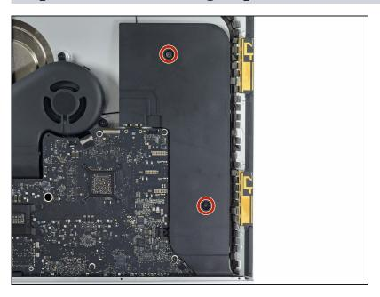
• Remove two 9.8 mm T8 screws.
