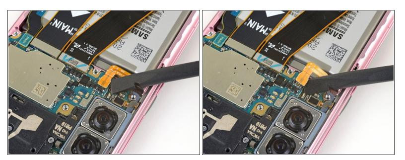
Use a spudger to pry up and disconnect the battery connector.
