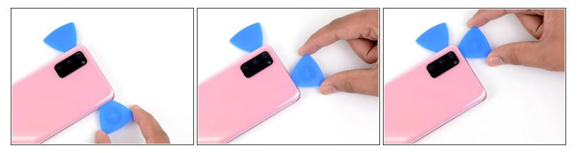
A The glass near the corners of the back cover is curved and very susceptible to cracking. Be gentle during this step to prevent damaging your back cover.
