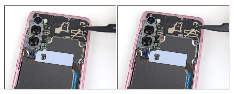
• Use a pair of tweezers to gently pull up and unclip the motherboard bracket from the plastic midframe.
