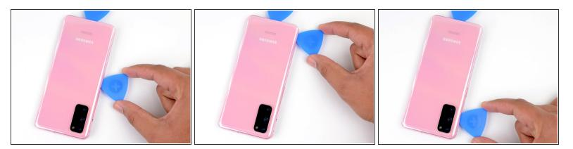
• Slide the pick all along the left edge of the phone to separate the back cover's adhesive.
