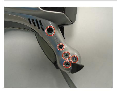
Remove the five screws on the drone's arms using a Torx T5 screwdriver.
