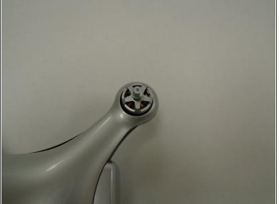
Holding the base of each propeller still, unscrew the propeller clockwise for each arm.
