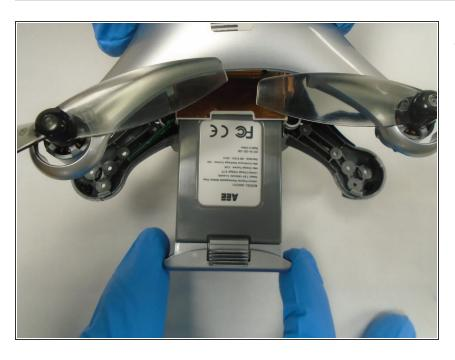
Take out and set aside the battery pack, located on the back of the AEE Mach 1.
