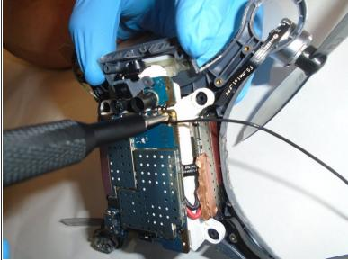
• Remove the four screws from each corner of the motherboard with a Phillips #00 screwdriver.
