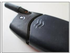
We'll start by flipping the phone with its back towards us and pushing on the top of the battery cover, then pulling down the cover as shown.
