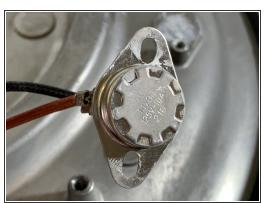
Remove two Phillips screws to detach the thermostat.
