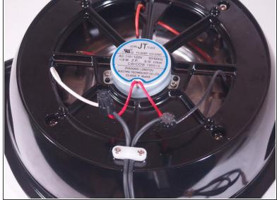
Removing the bottom cover exposes the internals of the popper. The base holds together the centrally mounted motor and the wires for the power cord and heating element.
