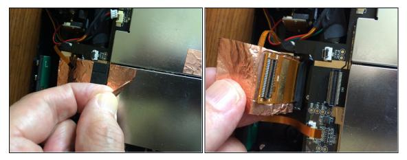
• Carefully peel back the copper foil covering the video connector until you can unmate it. Try not to tear the foil.
