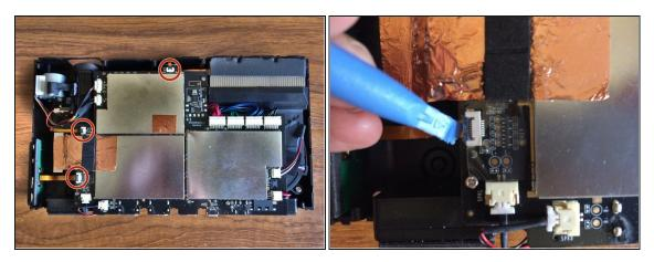
• Very gently lift the locking tabs on three ribbon connectors. A plastic prying tool is good for this. Withdraw the ribbons.
