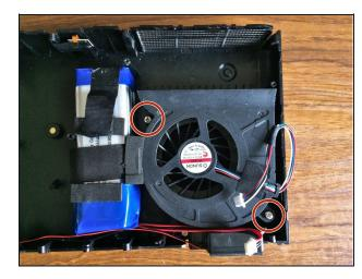
• Remove 2 screws securing the fan. This can now be lifted out allowing any dust build-up on th grill to be cleaned out.
