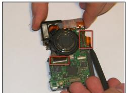
• There are two ribbon cables that must be unplugged before removing the assembly. To remove them, simply unsnap the jawbone connectors and then gently pull them out with either the <u>tweezers</u> or the spudger.
