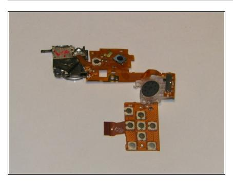
The rear control board should now be completely separate from the camera.
