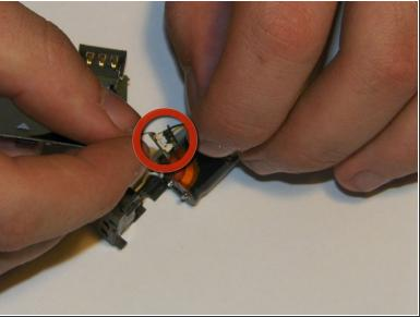
There is a small connector that mounts in the battery compartment that will need to be unplugged for the flash assembly to be fully removed.
