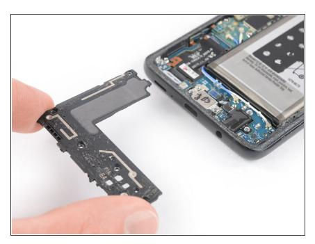
Remove the loudspeaker assembly.
