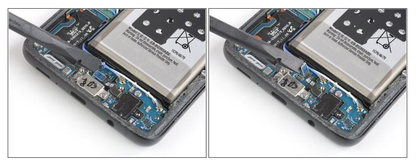
• Use the flat end of a spudger to pry up and disconnect the headphone jack flex cable.
