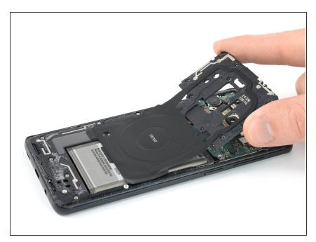
Remove the plastic cover containing the NFC antenna and the charging coil.
