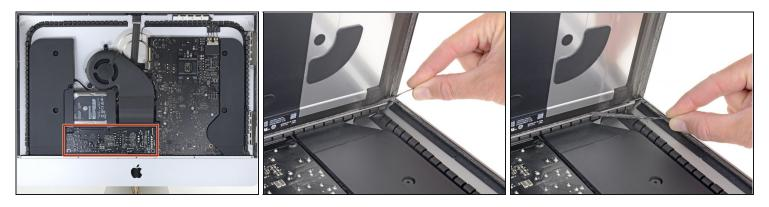
(i) If necessary, a <u>plastic card</u> can be used to cut any remaining sections of the bottom adhesive strip.
