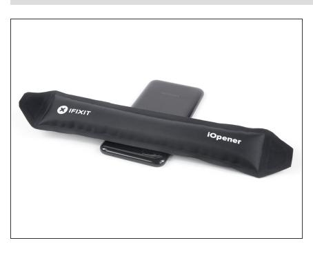
Apply a <u>heated iOpener</u> to the back of the phone where the fingerprint sensor is located to loosen the adhesive underneath. Apply the iOpener for at least two minutes.
