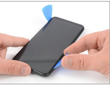
Slide the opening pick along the left side of the phone to release the plastic clips on the left side of the back cover.
