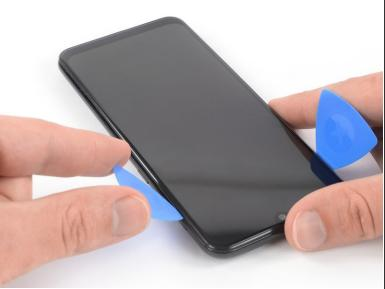
Slide the opening pick along the right side of the phone to release the plastic clips on the right side of the back cover.
