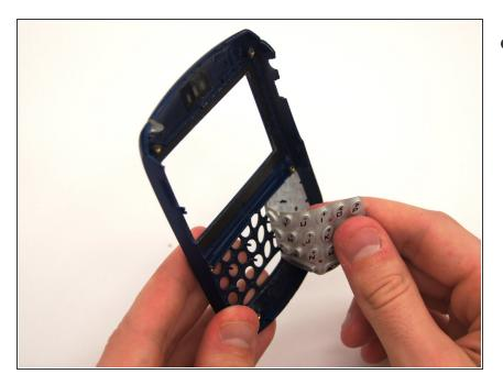
The keypad sits in the keyboard slots on the front cover. Simply peel the keyboard off and replace.
