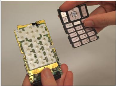
Carefully peel the rubber keypad mat off of the motherboard. The keypad is secured with an adhesive material, so there will be slight resistance.
