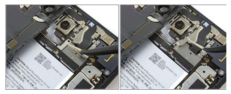
• Use a pair of tweezers to remove the back panel connector cover.
