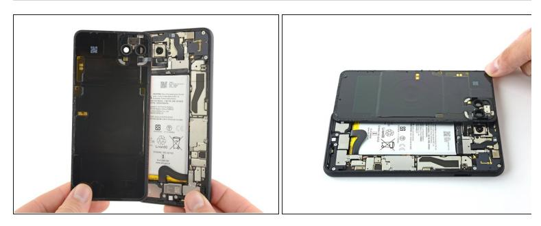
• Continue swinging open the back panel until you can rest it on the left edge the phone, being careful not to put any stress on the attached ribbon cable.
