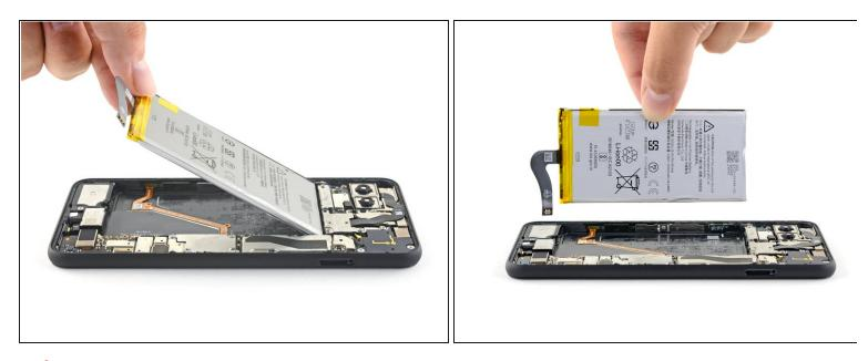
Don't reuse the battery if it has been deformed or damaged, as doing so is a potential safety hazard. Replace it with a new battery.
