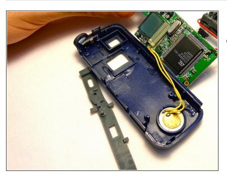
Carefully separate the grey side bar from the case and set it aside.
