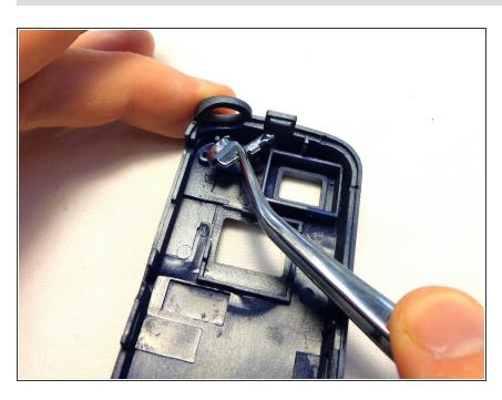
Use the tweezers to grasp the bottom of the capture button. Pull the capture button away from the case and set it aside.
