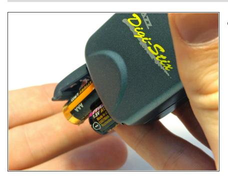
Tilt device so that batteries slide out.
