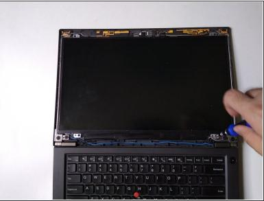
Use the Phillips #0 screwdriver to remove the four 3mm display screws.
