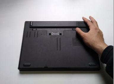
Slide each of the battery latches away from each other into the unlocked location.
