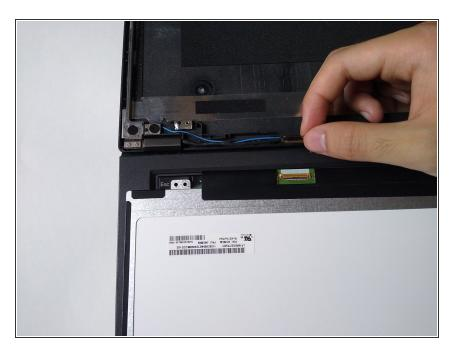
Gently remove the cable from the display by pulling it directly away from you.
