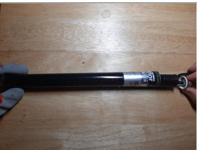
Without twisting or turning, slowly apply a pulling force to separate the glass tube from the core components of the water heater.
