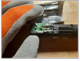
Hold the heating pad down to position the chip inside the housing. You may need to press the wires down to close the casing. Repeat this process again for the other cable.
