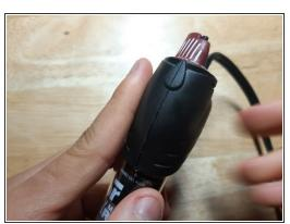
Reattach the plastic housing, making sure that the previously marked heating switch is properly aligned.
