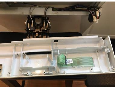
The circuit board sets in a gray plastic "sled". There are two tabs on the left that hold the circuit board onto the touchpad assembly. Move them to the left and pull up on the circuit board. It slides easily out from the left side, there are no tabs holding it.
