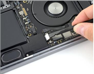
Disconnect the Touch Bar display cable by prying its connector straight up from the logic board.
