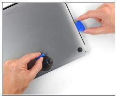
Repeat the previous step on the other side, using an opening pick to to release the second clip.
