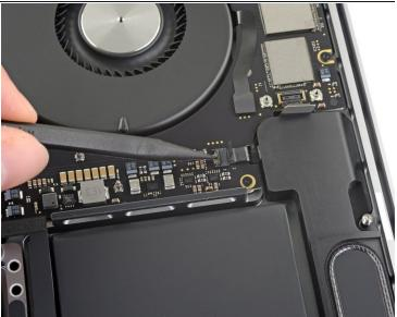
Open the locking flap on the right speaker cable's ZIF connector by prying it straight up from the logic board.
