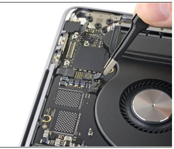
Peel back any tape covering the left fan connector.
