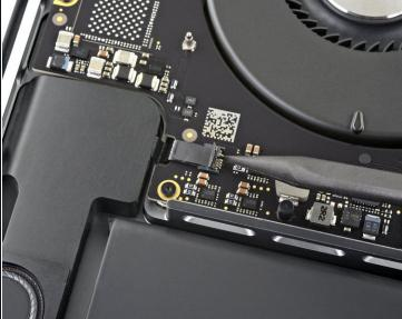
Open the locking flap on the left speaker cable's ZIF connector by prying it straight up from the logic board.
