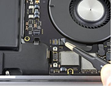
• Peel back any tape covering the first keyboard backlight cable connector.
