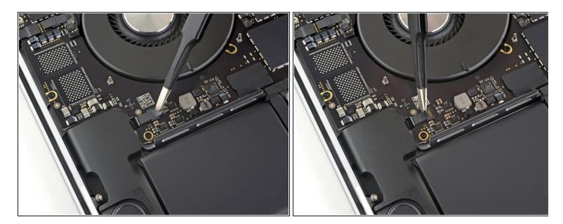
• Peel back any tape covering the left speaker cable connector.
