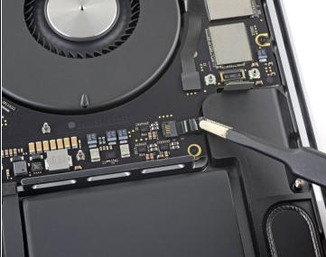
Peel back any tape covering the right speaker cable connector.
