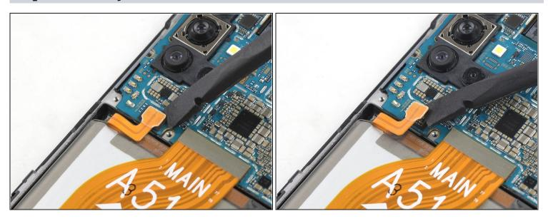
• Use the flat end of a spudger to disconnect the battery by prying the connector straight up from its socket.
