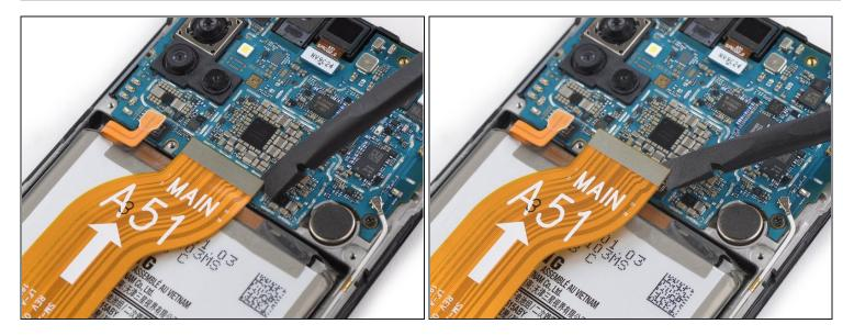
• Use the flat end of a spudger to pry up and disconnect the interconnect cable from the motherboard.
