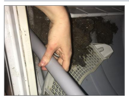
• Use an attachment to vacuum the remaining lint out of the trap.
