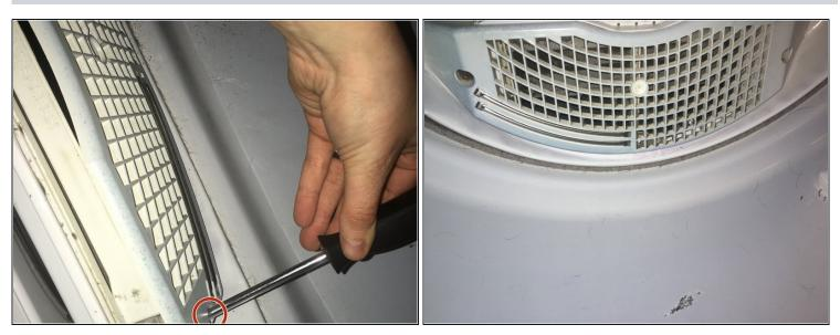
• Replace the lint trap and using the Phillips #0 screwdriver, screw the three 25.4 mm screws to secure the lint trap.
