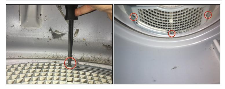
• Using the Phillips #0, remove three 25.4 mm screws that hold the lint trap to the dryer.
