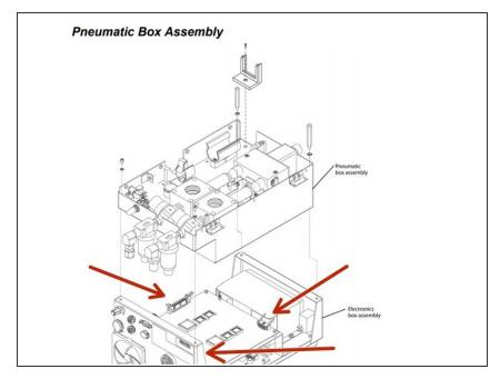
Remove cables from connectors J1, J2, J3, J4, J5, and J6 on the main PCB (4 connectors are not shown due to being blocked by the side panel). Note the position of these connectors for re-assembly.
