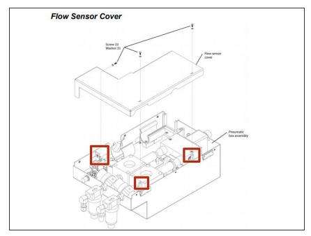
Remove the three screws and washers that secure the flow sensor cover to the pneumatic box assembly. Retain the hardware for re-assembly.
