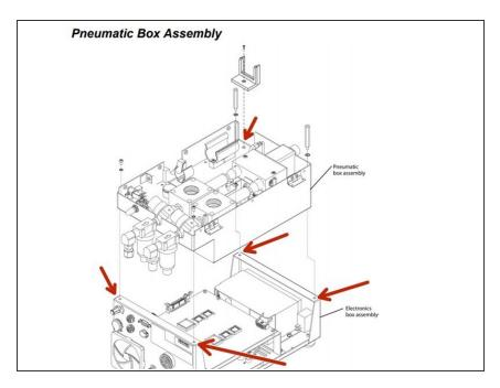
• Remove the two screws and washers (back corners), one screw and washer (exhalation module support bracket), and two standoffs and washers (front corners) that secure the pneumatic (upper) box assembly to the electronic box assembly. Lift the Pneumatics Box and carefully tilt to one side.
