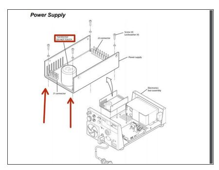
Lift the power supply out of the electronics box assembly.
