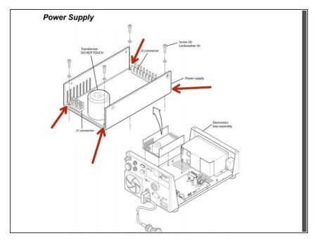
From the underside of the electronics box assembly, remove the four screws and lock washers that secure the power supply to the box assembly.
