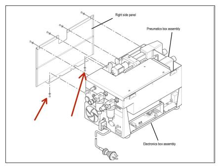
Remove the two screws and washers from the underside of the right side panel.
