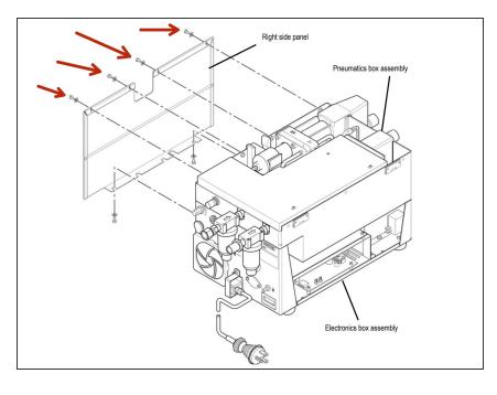
Remove the four screws and washers at the top edge of the right side panel.
