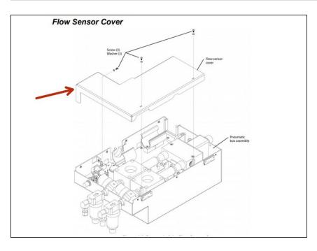
Remove the flow sensor cover.
