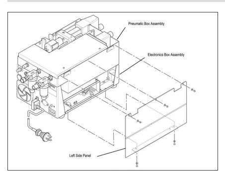
Remove the left side panel. Retain hardware for re-assembly.
