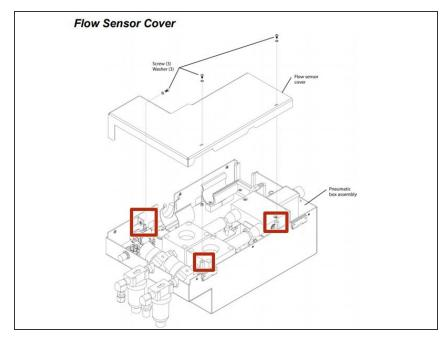
Remove the three screws and washers that secure the flow sensor cover to the pneumatic box assembly. Retain the hardware for re-assembly.
