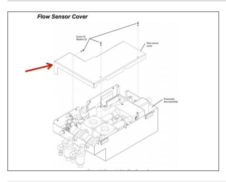
Remove the flow sensor cover.
