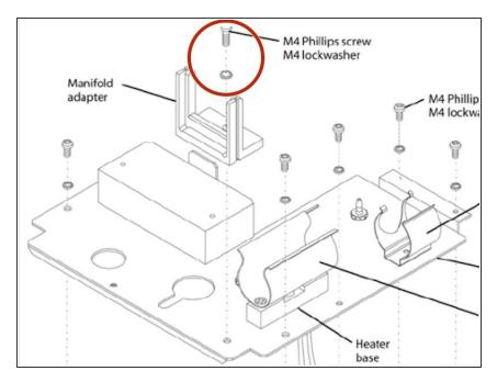
Remove the screw and washer that secure the exhalation manifold support to the pneumatic panel.
