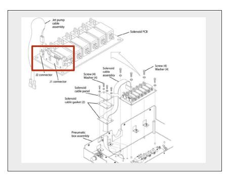
Remove the cables from J1 and J2 on the solenoid PCB.
