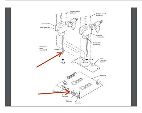
Disconnect the flow sensor cable from its 10 pin connector at the underside of the flow sensor PCB and lift out the flow sensor.
