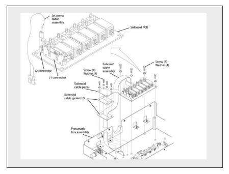
Carefully pull the tubes from their connections opposite the solenoid PCB (not directly from the solenoid PCB). Make note of the tubing connections for re-assembly.
