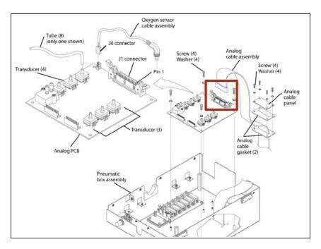
Remove the cable from the connector J1 on the analog PCB.
