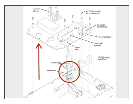
Lift the pneumatic panel out of the box, and from the underside, detach all tubes and the heater wires that connect to the analog PCB.
