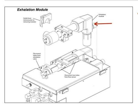
Pull the exhalation module straight up to remove it from the GDU.
