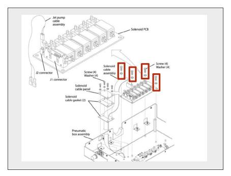
Remove the four screws and washers that hold the solenoid PCB to the pneumatic box assembly.
