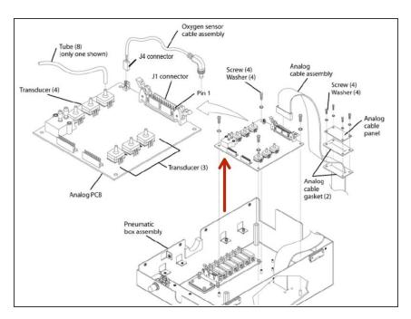
Hold tubing aside and remove analog PCB from the box assembly.
