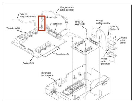
Disconnect the J4 connector from the analog PCB.
