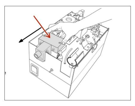
Slide the manifold/mixer assembly forward to disengage the flow sensors
