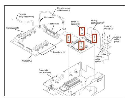
Remove the four screws and washers that hold the analog PCB to the pneumatic box assembly.
