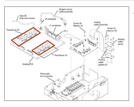
Carefully pull the tubes from each of the seven transducers on the analog PCB. Take note of the tubing connections for re-assembly.
