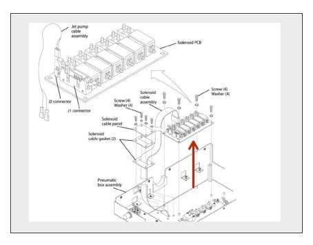
Hold the tubing aside and remove the solenoid PCB from the box assembly.
