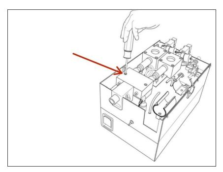
Remove the 2 screws and washers securing the manifold/mixer assembly
