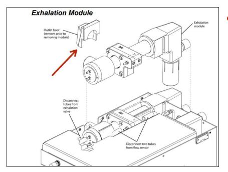
Pull up and remove the flexible rubber exhalation outlet boot (push fit).
