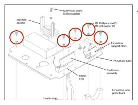
Remove the standoff and five screws and washers that secure the pneumatic panel to the pneumatic box.
