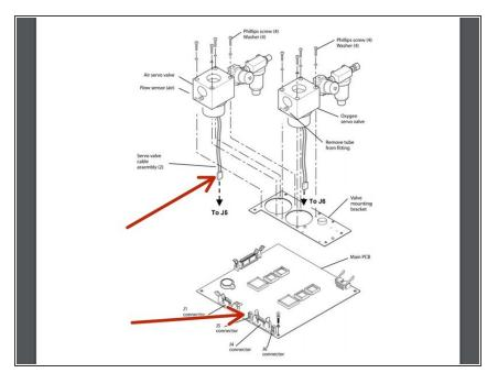
Disconnect the flow sensor cable from its 10 pin connector at the underside of the flow sensor PCB and lift out the flow sensor.
