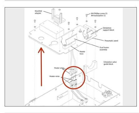
• Lift the pneumatic panel out of the box, and from the underside, detach all tubes and the heater wires that connect to the analog PCB.
