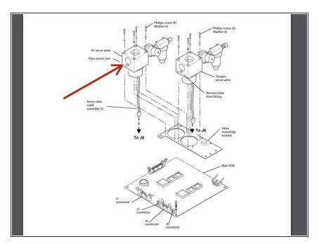
Gently pull each flow sensor straight out from the servo valve, (the flow sensor push-fits into the servo valve port).
