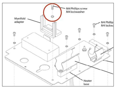
Remove the screw and washer that secure the exhalation manifold support to the pneumatic panel.
