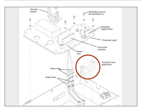
Pull up on the exhalation valve guide block to remove it from the pneumatic box.
