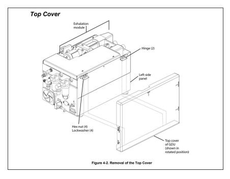
• Remove the cover and set aside. Retain hardware for re-assembly.
