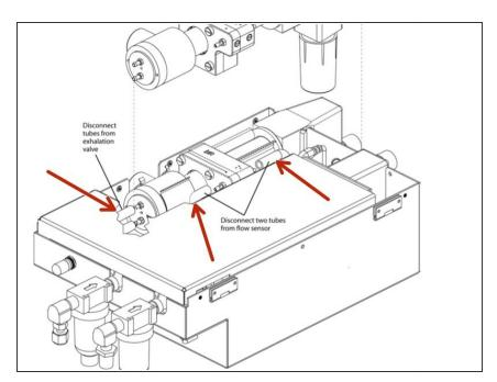
Disconnect the tubes from both sides of the flow sensor and the two tubes from the exhalation valve.
