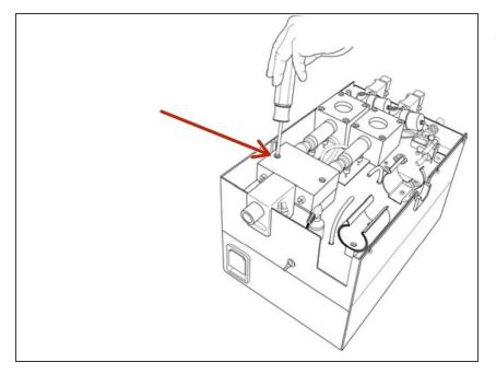
Remove the 2 screws and washers securing the manifold/mixer assembly
