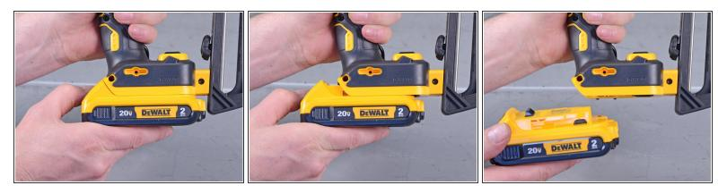
(i) Before you begin the repair, remove the battery from the device.
