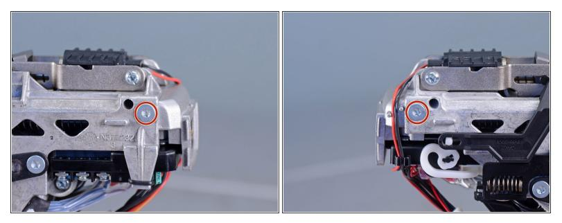
• Use a T20 driver to remove the two screws (one on either side) securing the back support .
