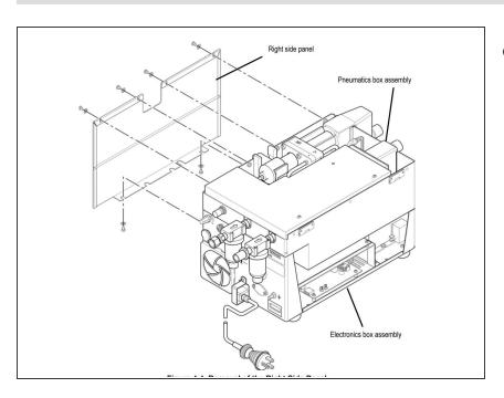
Remove the right side panel. Retain hardware for re-assembly.
