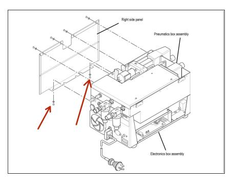
Remove the two screws and washers from the underside of the right side panel.
