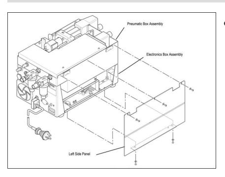
Remove the left side panel. Retain hardware for re-assembly.
