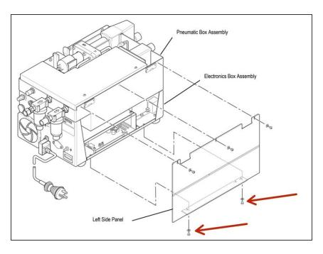
Remove the two screws and washers from the underside of the left side panel.
