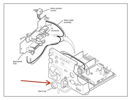
Unscrew the alarm retaining ring from the outside of the back panel; then pull the speaker from the inside of the back panel.
