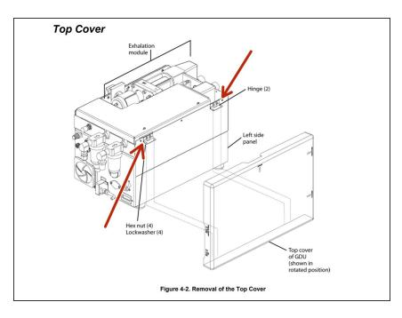
Remove the four hex nuts and lock washers (two at each hinge) that secure the cover to the hinges on the left side of the pneumatic box.
