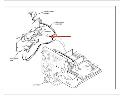
Disconnect the alarm cable assembly from P5 on the back panel PCB.
