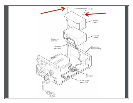
Remove the two nuts that hold the battery cover to the electronics box assembly and remove the cover.
