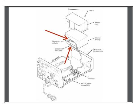
Disconnect the black and red wires from the battery terminals.
