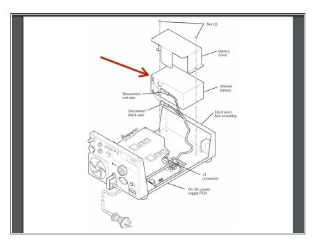
Pull the battery from the electronics box assembly.
