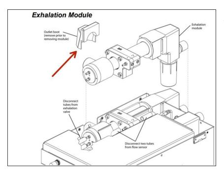
Pull up and remove the flexible rubber exhalation outlet boot (push fit).
