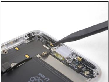
• Use the point of a spudger to gently pry the logic-board-side microphone free from the adhesive securing it in place.
