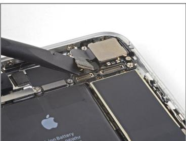
• Use the flat end of a spudger to disconnect the camera cable connector by prying it straight up from its socket.
