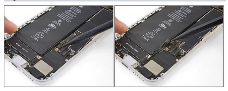
• Use the point of a spudger to pry up and disconnect the diversity antenna flex cable from the logic board.
