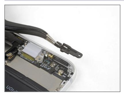
• Remove the barometric vent.
