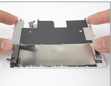
Gently lift the LCD shield plate from the display assembly.
