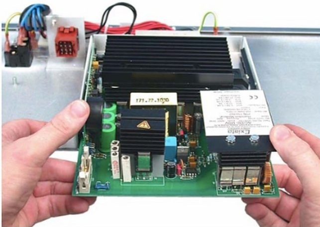
Figure 11-202. Sliding the power supply from its housing
