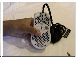
Replace the two Phillips #0 screws in the mouse's housing.
